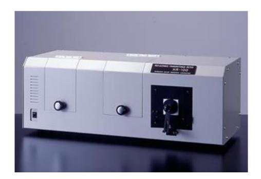
The HR-100 is designed to measure total light transmittance, diffuse light transmittance, and haze. It is ideally suited to make these measurements for light transmissible materials such as plastics, films, glass and liquid as well as light reflective materials with a high degree of specularity such as metals, coating and mirrors.
